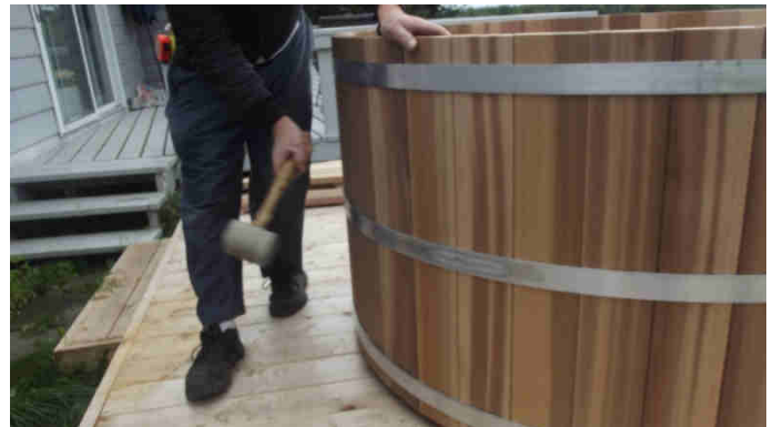
Fig. 9.2 Hitting straps hard all around while tightening.
