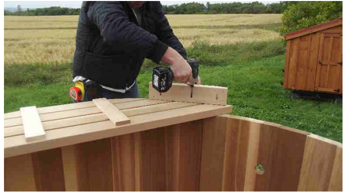
Fig. 10.1.1 Rest the benches on top of the tub to attach the bench-end supports
